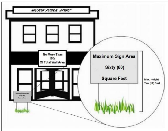
Figure 16.6.1. Front Yard Signage
