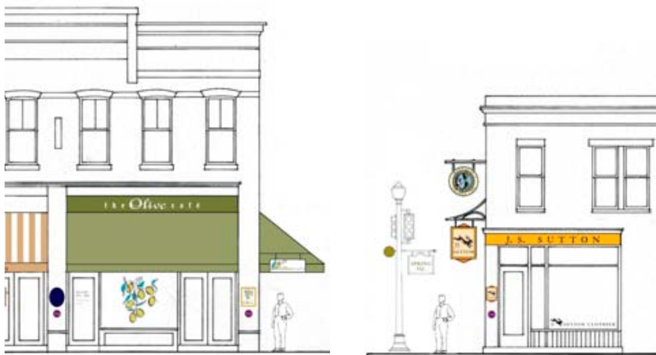
Awnings are often used for identity signs. etching on shopfronts and Blade signs are also used in combination
